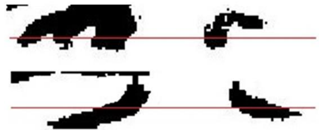
Fig. 5: The ratio of black pixels in upper part of the image of eye to the black pixels in lower part while eyes are open (upper section) and closed (lower section)
