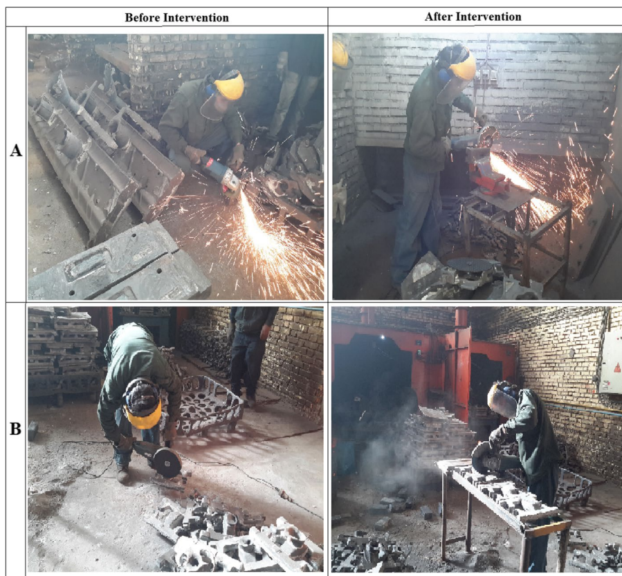
Fig. 2 Some workstations before and after intervention. A Grinding worker for large parts; B Grinding worker for small parts
