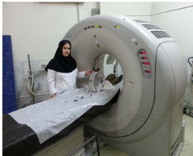
Fig 2. The use of CT bed and phantom to test the correct function
