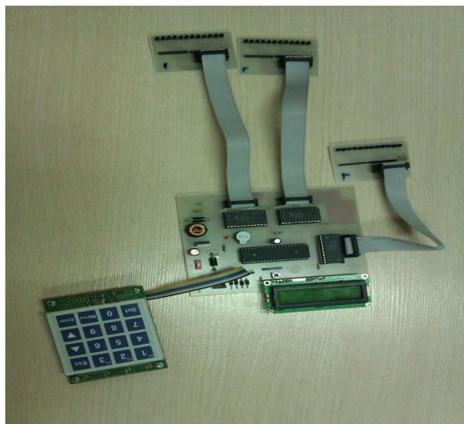
Fig 1 . The keyboard and receiver circuit microcontroller with light emitting diodes
